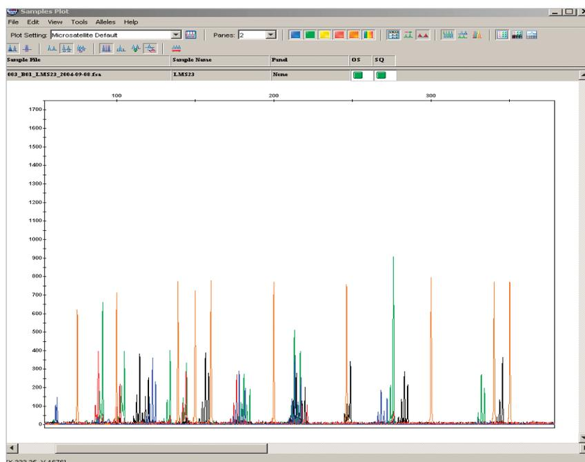
Figure 3. Five-dye chemistry increases the number of markers that can be run in a single capillary, for improved throughput. Above is an example of 18 microsatellite loci co-electrophoresed in a single capillary.
