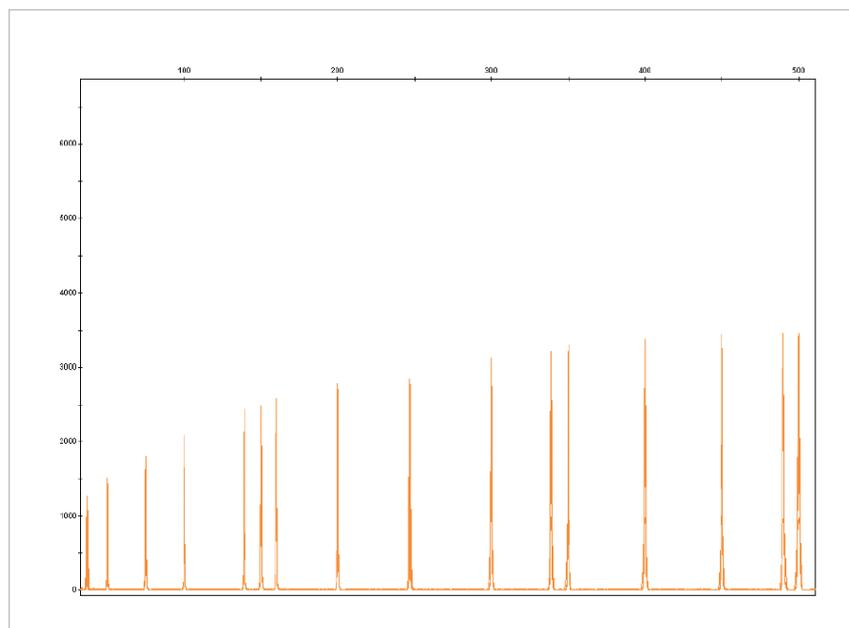
**Figure 4.** Overlay of 16 GeneScan™-500 LIZ® size-standard electropherograms shows sizing precision on the 3130 Series Systems.
